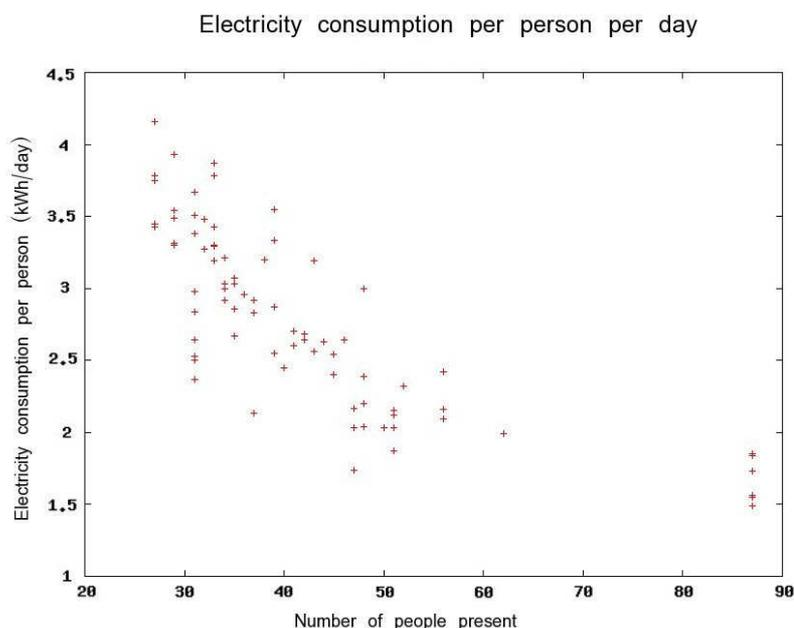
**Figure 4: Electricity consumption per person per day as a function of the number of people using the system**
