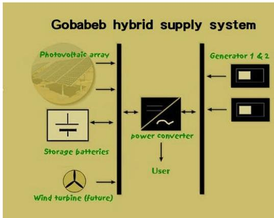
**Figure 2: Gobabeb's hybrid electricity supply system**
